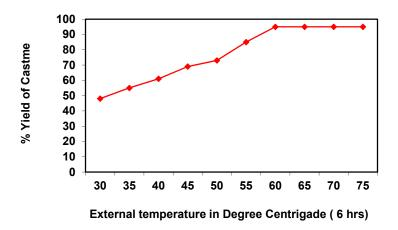
Fig. 7. Effect of external temperature on the reaction course
