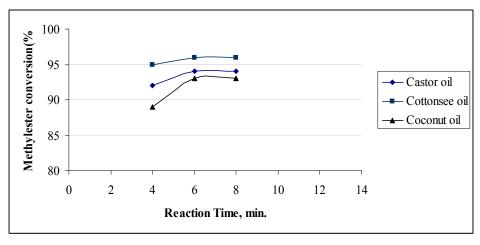
Optimum Reaction time = 6min.
