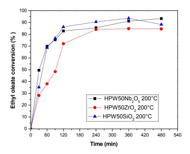
Reaction conditions: oleic acid (1.0 mmol); ethanol (155.0 mmols); catalyst (50.0 mg); 60 °C
