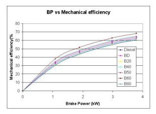
Fig. 17. Comparison of brake power and mechanical efficiency
