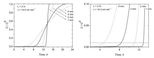
Fig. 7. Adsorption of glycerol from biodiesel. Breakthrough curves as a function of pellet diameter ( $d_v$ ). Breakthrough condition  $C/C^0$ =0.01, L=2 m, U=14.4 cm min<sup>-1</sup>.
