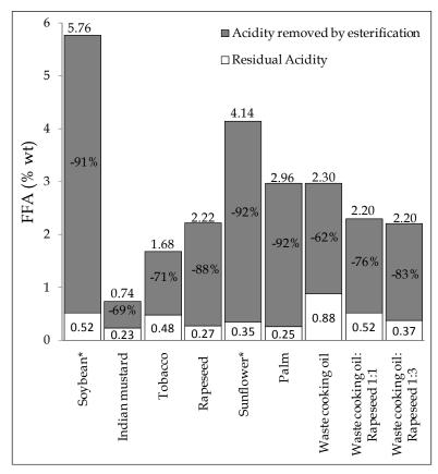
Fig. 3. Acidity removed by esterification (6 hr) and residual acidity of different oils used as raw material: slurry reactor, T=338K, catalyst: Amberlyst® 46 weight ratio methanol/oil=16:100, weight ratio catalyst/oil=1:10; \*commercial, refined oils with the addition of pure oleic acid.
