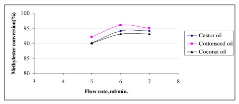
Optimum flow rate = 6ml/min
