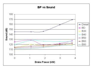
Fig. 23. Comparison of brake power and sound
