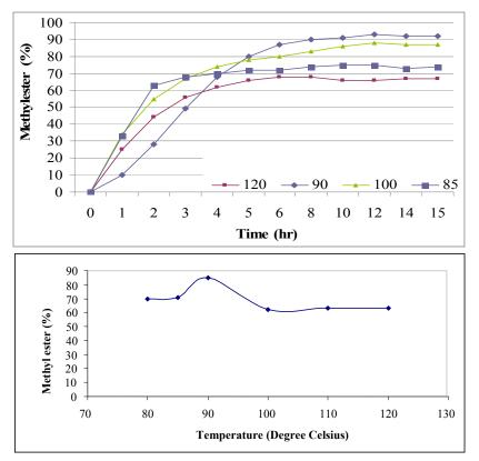
Fig. 19. The effect of the reboiler temperature on methyl esters content in product
