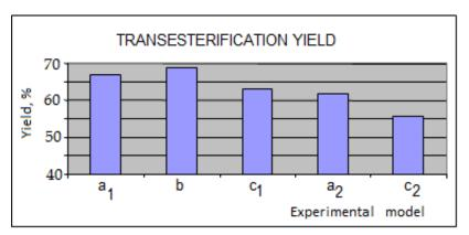
Fig. 8. The vegetable oils transesterification yield for the 3 experimental models: a<sub>1</sub>-batch model without solvent, with soya oil; a<sub>2</sub>-batch model without solvent, with rapeseed oil; b-semibatch model without solvent, with soya oil; c<sub>1</sub>-batch model in hexane with soya oil; c<sub>2</sub>-batch model in hexane with rapeseed oil
