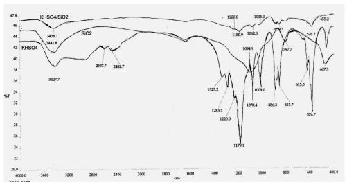
Fig. 6. FT IR spectra of pure KHSO<sub>4</sub>, Pure SiO<sub>2</sub> and KHSO<sub>4</sub> supported on SiO<sub>2</sub>
