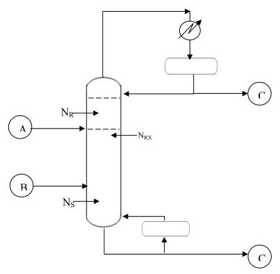
Fig. 4. Flow sheet of ideal reactive distillation column
