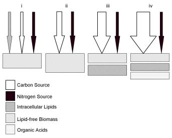
Fig. 6. Metabolic activity of oleaginous fungi (e.g. *Y. lipolitica*) as a function of carbon flow rate for a fixed nitrogen flow rate. Arrows indicate the consumption of nitrogen and carbon sources by the cells; squares indicate production rate. The dimension of arrows and squares is proportional to flow. (adapted from Beopoulos et al., 2009a)
