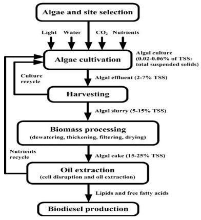
Fig. 5. Microalgae biodiesel value chain stages.
