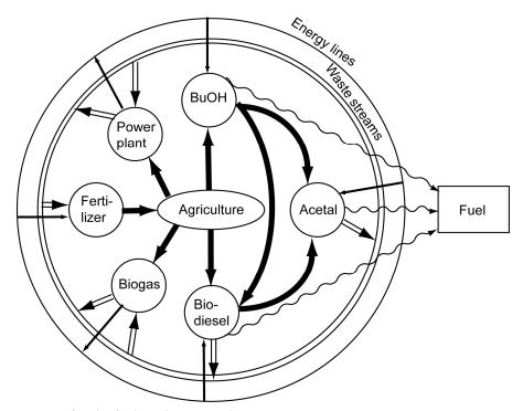
Fig. 1. Waste free biofuel production cycle
