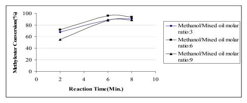
Fig. 9. Effect of Methanol to Mixed oil Molar ratio on methyl ester conversion
