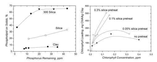
Fig. 1. Isotherms of adsorption of phosphatides on silica (left). Adsorption of chlorophyll on clay as a function of the silica adsorption pretreatment (right). Welsh et al. (1990).
