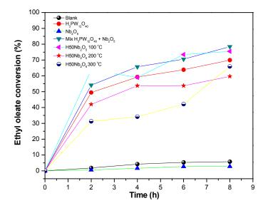
Reaction conditions: catalyst (50.0 mg); oleic acid (1.0 mmol); ethanol (155.0 mmols); 60°C.
