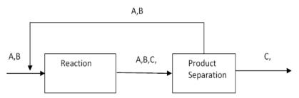
Fig. 2. Standard process scheme for reversible reactions in which the conversion is limited by the chemical equilibrium [9]
