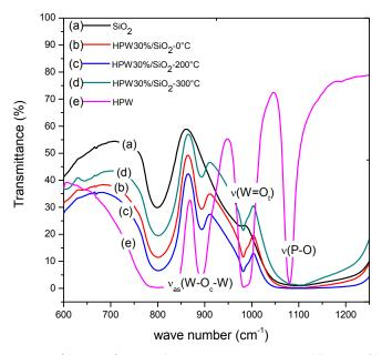
Fig. 2. FTIR spectra of (30 %w/w HPW)  $H_3PW_{12}O_{40}$  composites (a)- SiO<sub>2</sub>; (b)- HPW 30%/SiO<sub>2</sub>-100°C; (c) HPW 30%/SiO<sub>2</sub>-200°C; (d) HPW 30%/SiO<sub>2</sub>-300°C; (e)- HPW.
