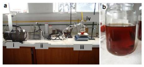
Fig. 10. Biodiesel distillation (a) Mounting: i. vacuum pump ii. Vacuum trap iii. Hot plate iv. Thermometer (b) Distilled biodiesel
