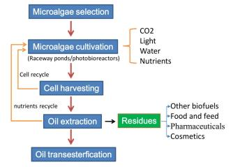
Fig. 5. Microalgal biodiesel production pipeline
