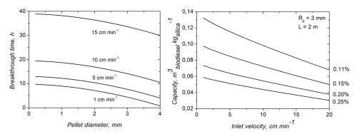
Fig. 8. Adsorption of glycerol from biodiesel. Left: breakthrough time as a function of U and  $d_p$  (L=2 m, U=14.4 cm min<sup>-1</sup>). Right: influence of U and  $C^0$  on the processing capacity ( $d_p$ =3 mm, L=2 m).
