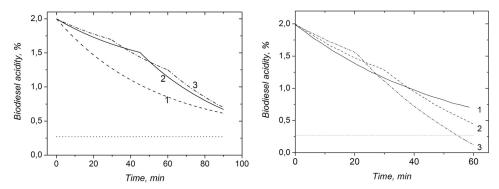
Fig. 9. Biodiesel acidity as a function of time and the number of countercurrent tank bleaching steps (1, 2 and 3) (Manuale, 2011). Adsorbent load=2%, initial biodiesel acidity=2%,  $K_{LDF}$ = 0.0188 min<sup>-1</sup>. Left: Linear adsorption (Henry's law, H=37.6). Right: Irreversible adsorption (square isotherm). Dotted line: FFA European standard EN 14214, FFA limit.
