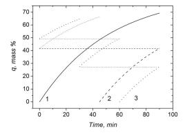
Fig. 10. Adsorbent load as a function of time and the number of countercurrent bleaching steps (1, 2 and 3) (Manuale, 2011). Process conditions as in Figure 9.
