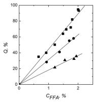
Fig. 2. Adsorption isotherm for silica TrySil 3000 at three different temperatures (Manuale, 2011). 70 °C ( $\blacksquare$ ), H=44.6. 90 °C ( $\bullet$ ), H=31.4. 110 °C ( $\triangle$ ), H=18.3.  $\triangle H$ =-5.7 kCal mol<sup>-1</sup>.
