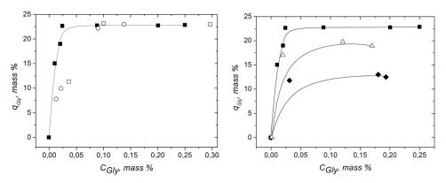
Fig. 3. Adsorption of glycerol over silica (Mazzieri et al., 2008). ( $\blacksquare$ ) Pure biodiesel. ( $\square$ ) Biodiesel spiked with water (944 ppm). ( $\circ$ ) Biodiesel spiked with soap (270 ppm). ( $\Delta$ ) Biodiesel spiked with MG (7500 ppm). ( $\bullet$ ) Biodiesel spiked with methanol (12000 ppm).
