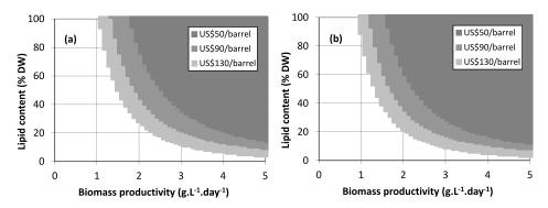
Fig. 2. Lipid contents and biomass productivities required for economic feasibility in (a) large-scale, outdoor raceway ponds and (b) large-scale, outdoor photobioreactors. Dark grey region: productivities economically feasible at US\$ 50 per barrel crude oil (cost of algal oil per L lower than cost of regular diesel per L). Additional region for crude oil price US\$ 90 per barrel = mid-grey and US\$ 130 = light grey
