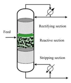
Fig. 1. The general configuration of Reactive Distillation
