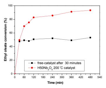
Reaction conditions: catalyst (50.0 mg); oleic acid (1.0 mmol); ethanol (155.0 mmols); 60°C.
