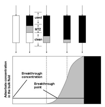
Fig. 5. Adsorption colum zones. Relation to breakthrough curve.
