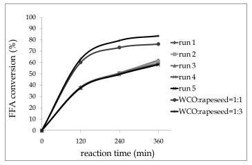
Fig. 4. FFA conversion (%) vs reaction time of waste cooking oil (WCO) and its blends with rapeseed oils: slurry reactor, T=338K, catalyst: Amberlyst® 46 weight ratio methanol /oil= 16:100, weight ratio catalyst/oil=1:10.
