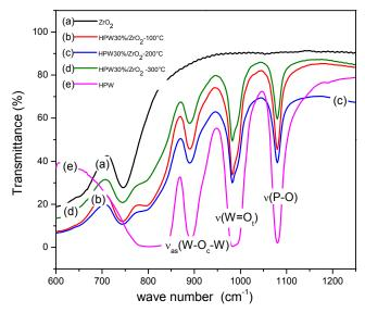
Fig. 3. FTIR spectra of  $H_3PW_{12}O_{40}$  (30% HPW) composites (a)- ZrO<sub>2</sub>; (b)- HPW/ZrO<sub>2</sub>-100 °C (c) HPW 30%/ZrO<sub>2</sub>-200°C; (d) HPW 30%/ZrO<sub>2</sub>-300°C; (e)- HPW.
