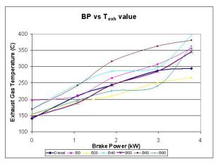
Fig. 14. Comparison of brake power and exhaust gas Temperatur
