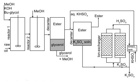
Fig. 2. Flow-sheet of biodiesel synthesis
