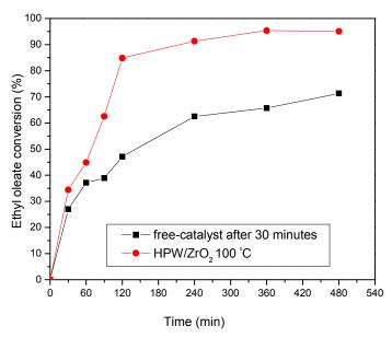
Reaction conditions: catalyst (50.0 mg); oleic acid (1.0 mmol); ethanol (155.0 mmols); 60 °C
